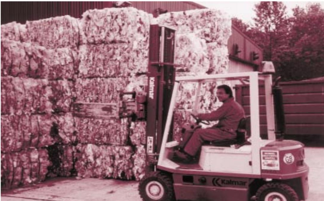
Baled cans ready for recycling. Recycling aluminium saves up to 95% of the energy used to produce virgin aluminium. *Photo: New Forest District Council.*
